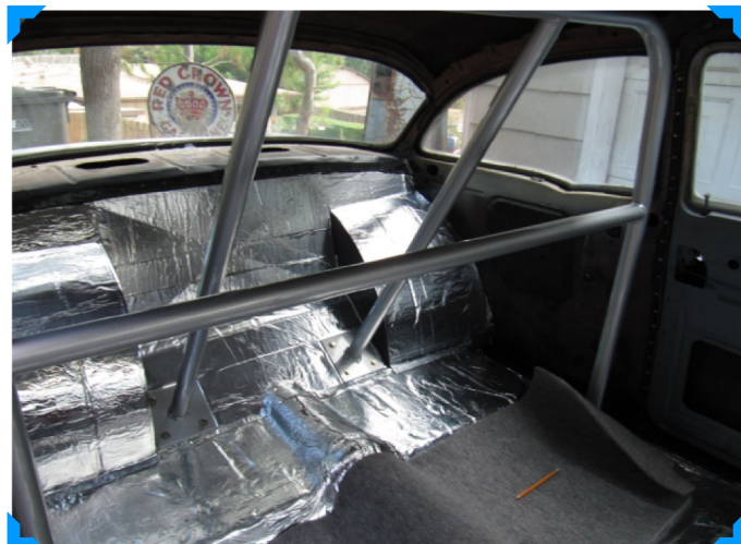
Ava and Annette moved in to place Fat Mat heat and sound deadening material. With any work operation it's important to assume a comfortable work position.
