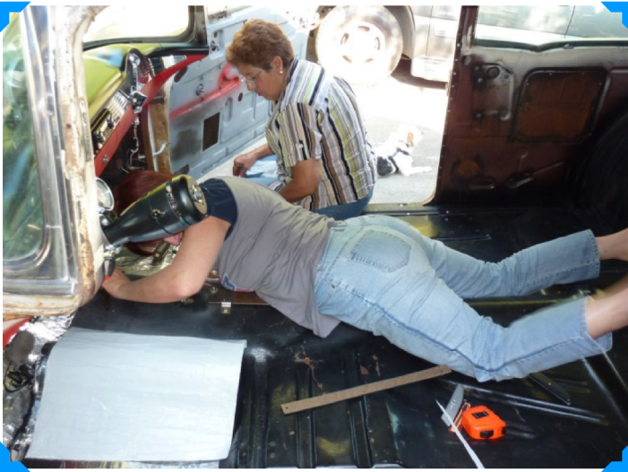
Ava and Annette moved in to place Fat Mat heat and sound deadening material. With any work operation it's important to assume a comfortable work position.
