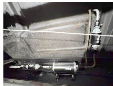
Sen Fuel Filters and Fuel Pump Installed
