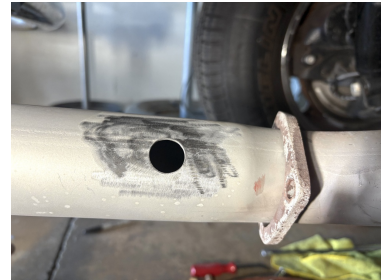
Hole Drilled in Exhaust Pipe
