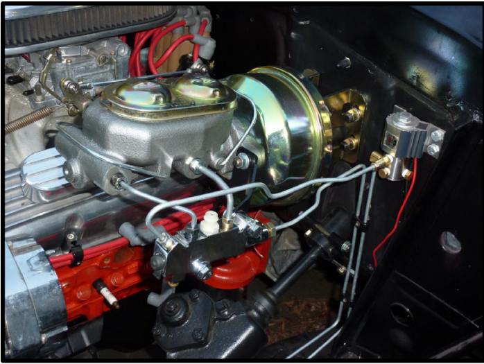
The master cylinder/booster has been bolted to the firewall as well as a Hurst line lock.
