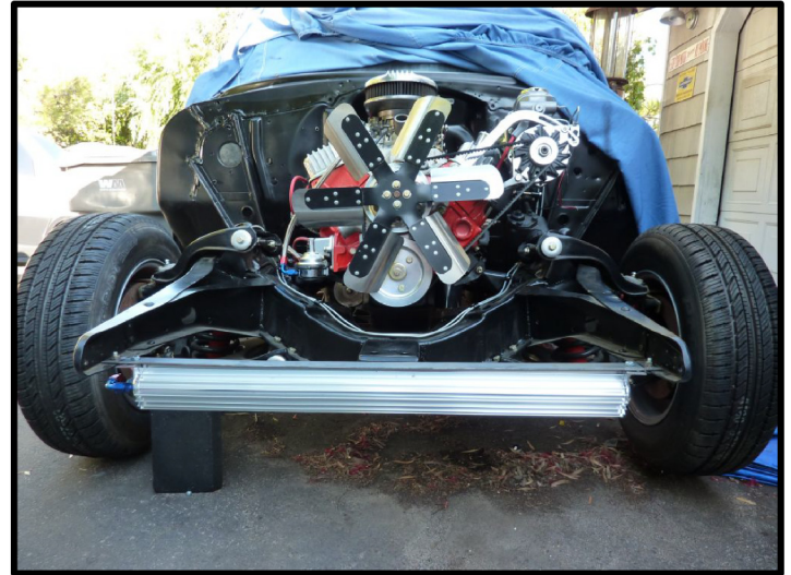
An extruded aluminum dual pass transmission cooler has been mounted between the front frame horns and will be tucked behind the front bumper.
