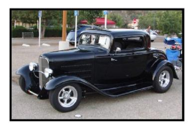
It is a 1932 Ford 3 window coupe that was built in 2012 and I bought it with just 700 miles on the odo. It has a Chevy 350 roller rocker crate motor, Chevy 350 turbo tranny and a Ford 9" rear end. Coil overs all the way around, discs in front, drums in the rear. Vintage air. It is a Kilborne glass body, top chopped 3", and the running boards and hood are steel.
