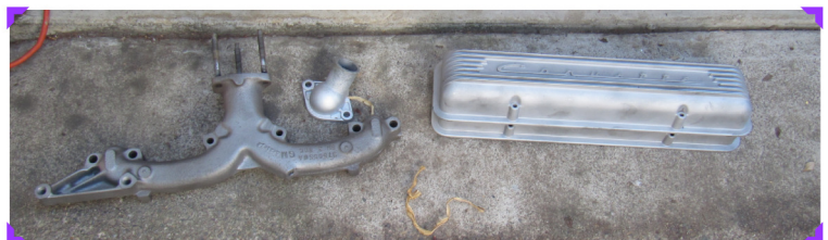
Bob Brown visited the Bishops' blast cabinet to bead blast his valve covers, exhaust manifold and thermostat housing to give them a fresh matte finish.
