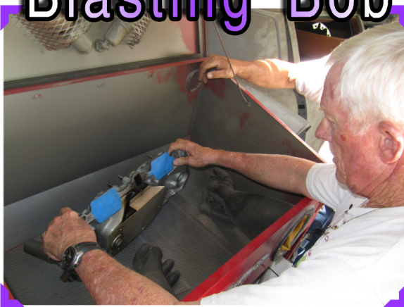
Bob Brown visited the Bishops' blast cabinet to bead blast his valve covers, exhaust manifold and thermostat housing to give them a fresh matte finish.
